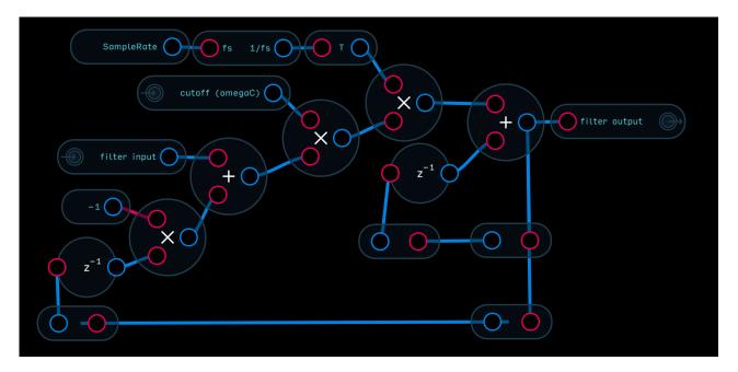
Note that the patch contains two unit delays, one is part of the integrator and the other for the previous sample that is added to the integrator. Since both z-1 nodes are attached to the integrator output, they both have the same value so we can simplify the patch by removing one of the unit delays. It would also be possible to condense the Add and Multiply nodes into a single Expression node, but this approach more clearly demonstrates the visual nature of programming in Audulus.
