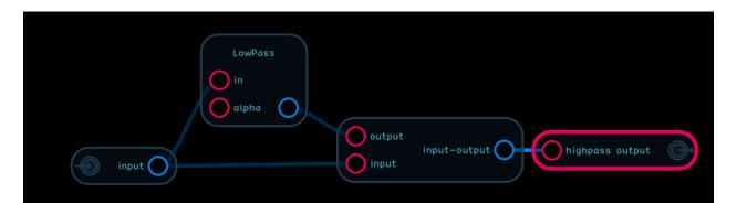
Of course it's simpler to use the built-in HighPass node. As mentioned earlier, both of these nodes are first order filters and they have a cutoff slope of 6dB per octave which is not very steep. They are very efficient however and are a good choice for many filtering applications.
