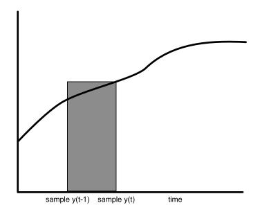
This is okay as long as T is small compared to the rate of change from sample to sample, or to put it another way, so long as the maximum frequency is much less than the sample rate.
