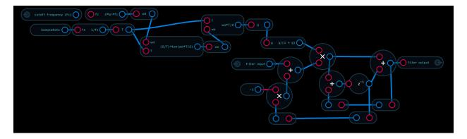
This is the completed digital model of the analog RC low pass filter we diagrammed at the beginning. It's also how the built-in LowPass filter node in Audulus works internally. Since the built-in node is somewhat more efficient than our module, it's generally preferable to use the built-in node.
