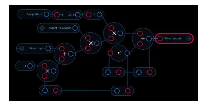
This is the simplest implementation of a first order low-pass filter, however it isn't a particularly good one. As we saw in the analog filter, when we integrate a function we are calculating the area under the curve of the function. Our current approach takes the value of sample t and multiplies it by the sample time T. This calculates a rectangular area.
