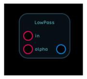
What's alpha? Alpha is another way to represent the cutoff frequency of the filter. For use with Audulus alpha is calculated as: 1-(fc\*2\*pi)/(fs+fc\*2\*pi) where fs is the sample frequency and fc is the cutoff frequency. Note in some references you will find alpha defined as (fc\*2\*pi)/ (fs+fc\*2\*pi) instead. The high pass node is similar to the low pass node. In fact, if you subtract the output of the low pass node from the input to the node, you will have a high pass filter.
