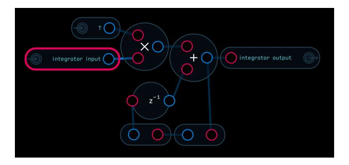
This takes an input value, adds the previous output value and sends it to output. We know that the sample rate for Audulus is 44.1 kHz so the time for each sample is 1/sample rate or in Audulus:
