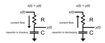
Because the resistor and capacitor form a voltage divider, when the input voltage is changing, only a portion of the input signal appears at the output. This smooths out the fluctuations in the input signal.
